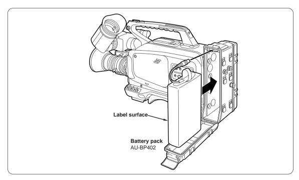
**CAUTION:** The unit's power must be turned off before the plug is connected or disconnected.
